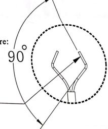
Adjust the front end of the clip with tweezers to make the angle close to 90 degrees.
