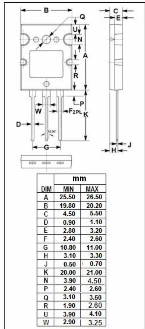
**SPTECH Silicon NPN Power Transistor**
