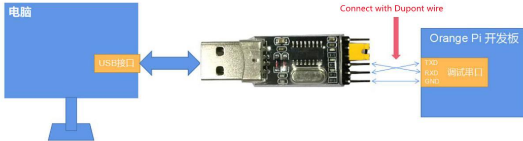
Schematic diagram of connecting the USB to TTL module to the computer and the Orange Pi development board
