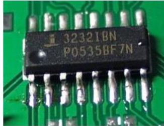
Too much solder
