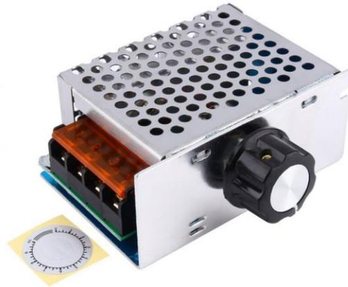
This is a 4000W Thyristor SCR Voltage Regulator Temperature Dimmer for Speed / Light (AC 220V). 4000W Thyristor SCR Voltage Regulator is SCR Dimmer which can be used to control 220V Appliances. It can be used as a light dimmer, fan speed controller, stove temperature controller. It is easy and simple to use and can control appliances up to 4000W
